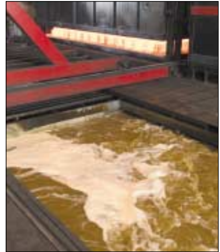
The bath is formulated at 15% to 17% concentration. This high molecular weight polymer quenchant was engineered for high alloy steels, and applications where distortion control is critical.
